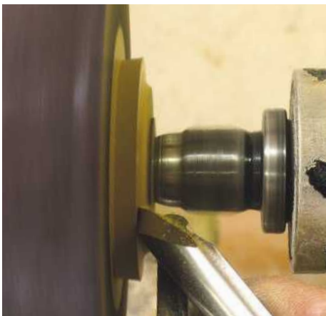
▲ Pic.19 The spindle gouge is used for this cut, but make sure that the bevel of the tool is lined up in the direction of the cut. If the point touches the wood it will run back on you
